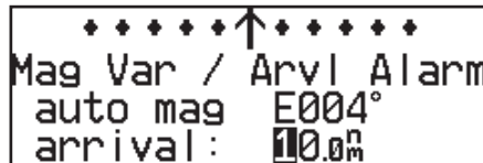
Setting the arrival alarm to 10 nautical miles.
