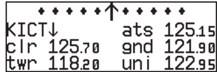
Airport communication page. The down arrow next to the identifier indicates additional frequencies may be displayed by rotating the ● knob.
