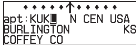
Entering a waypoint by identifier.
