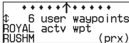
User waypoint list showing the current active-to waypoint and a proximity waypoint.
