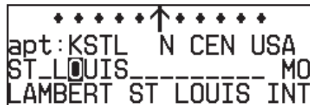
Entering a waypoint by city. Note that punctuation marks are not used when entering locations or names. Use spaces, where appropriate, to identify these marks. For example, St. Louis would be entered as "ST LOUIS" without a period.
